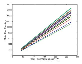
Figure 2. Meter raw reading before calibration
