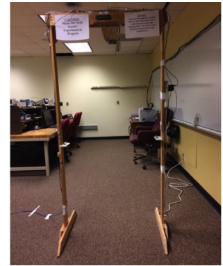
(c) Front view of the door frame with the ultrasonic sensors mounted.
