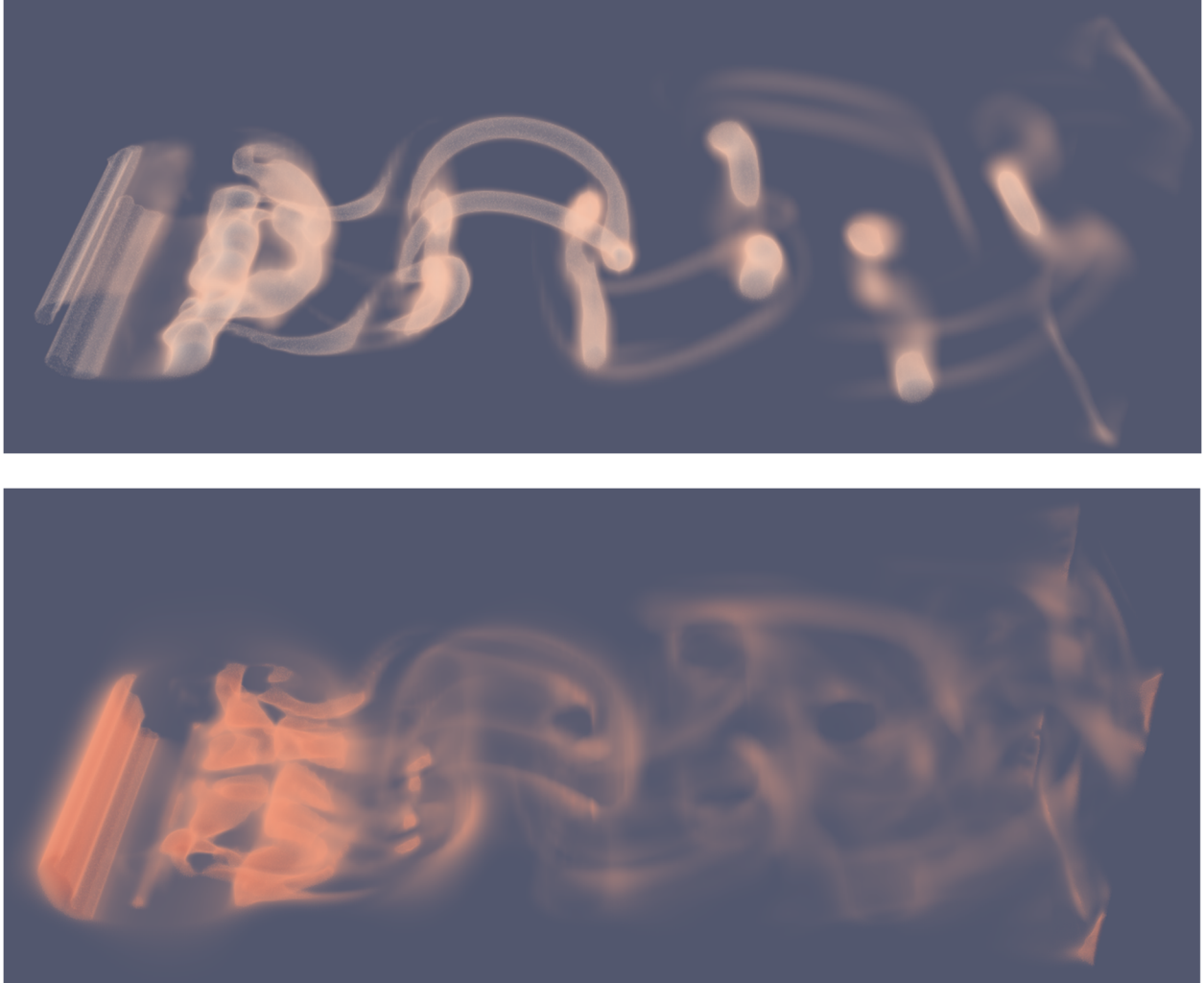
Figure 4. Two volume renderings using two different sets of transfer functions. The top image shows the tube-like small structures in the data, while the bottom image shows the larger structures.
