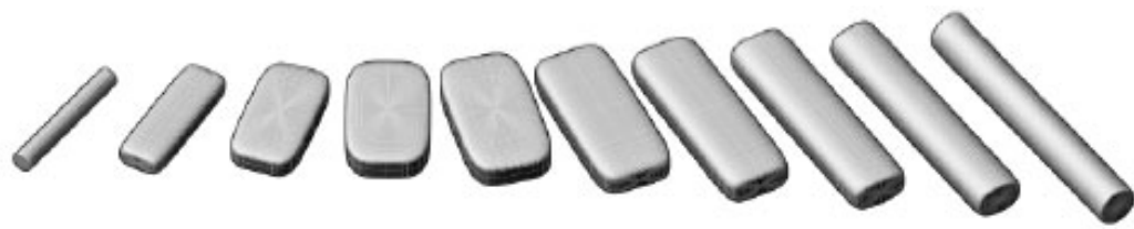
(a) Linear interpolation of tensor components: (1 - t)T_1 + tT_2
