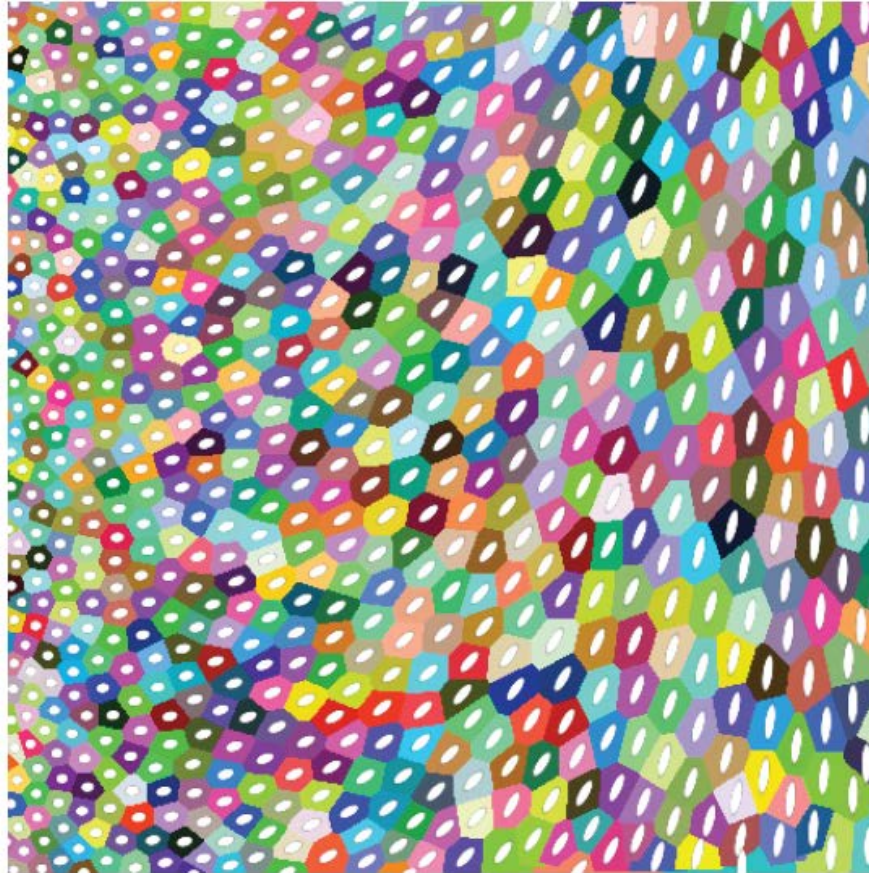
Fig. 7. Anisotropic Voronoi cells resulting from the simplified distance measure. The grid used for relaxation has a resolution of 512 \times 512 .
