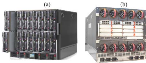
Fig. 7 BladeSystem c7000 enclosure (a) front view, (b) rear view
