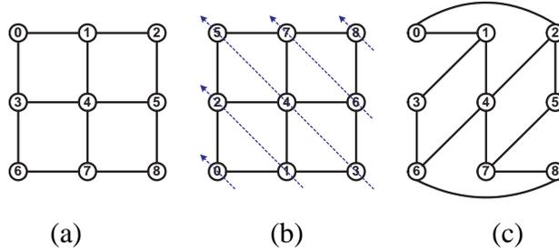
**Figure 1. 2D grid topology with row major and diagonal process numbering**
