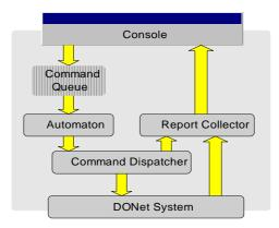
Fig. 6. A modular architecture of the experiment system.
