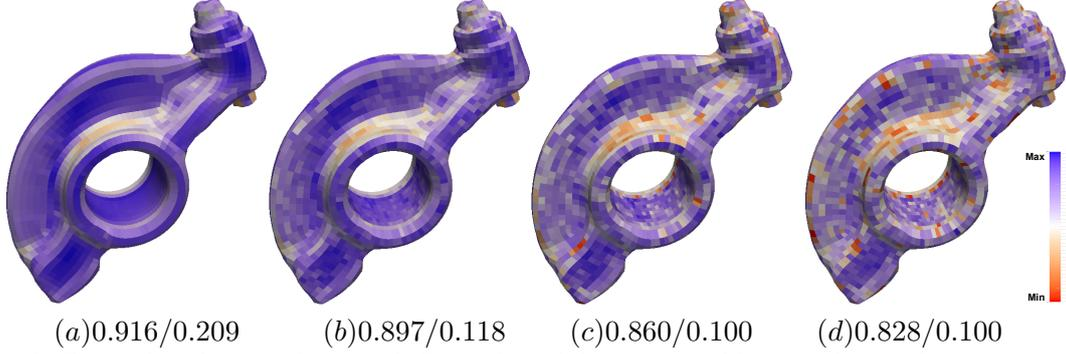
Figure 1: Original rocker arm hex-mesh from [3] and the generated hex-meshes with varying quality.
