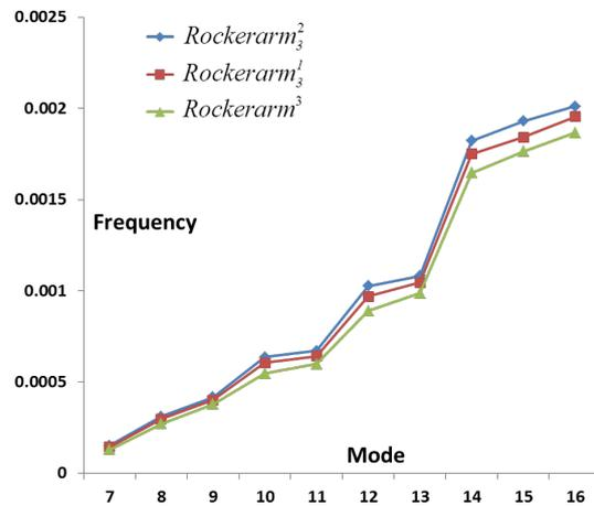
Figure 4: Comparisons among the eigenvalues corresponding to various modes for three rocker arm meshes.
