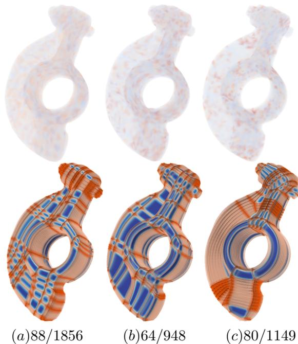
Figure 5: Rocker arm hex-meshes produced by (a-b) [4] and (c) [3]. First row shows the displacement distribution, second row shows the corresponding singularity-structures for them. The numbers of singularity nodes and the patch numbers of the singularity-structures for these meshes are 88/1856, 64/948, 80/1149, respectively.
