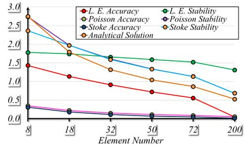
**Figure 1:** Both the accuracy and the stability of the elliptic PDE problems are improving as the element number of the cube hex-mesh increases. X-axis is the element number of a hex-mesh. Y-axis is either  $\lambda_{\min}$  for the accuracy of a solution,  $\log(\lambda_{\max})$  for the stability of a solution, or the true value of the “Analytical Solution”.
