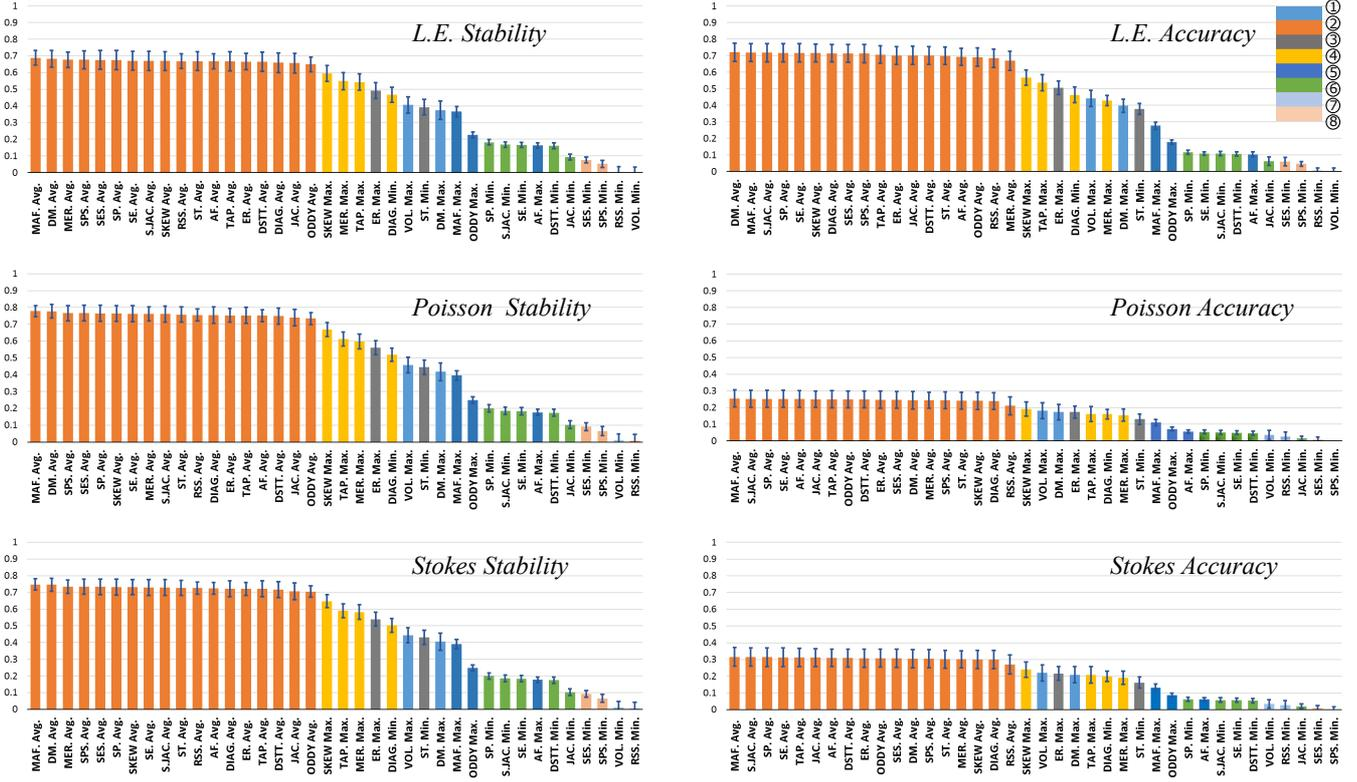
**Figure 8:** Metrics are ranked based on their correlations with the Stability (left column) and Accuracy (right column) measurements of the linear elasticity problem, Poisson’s problem, and Stokes problem, respectively.
