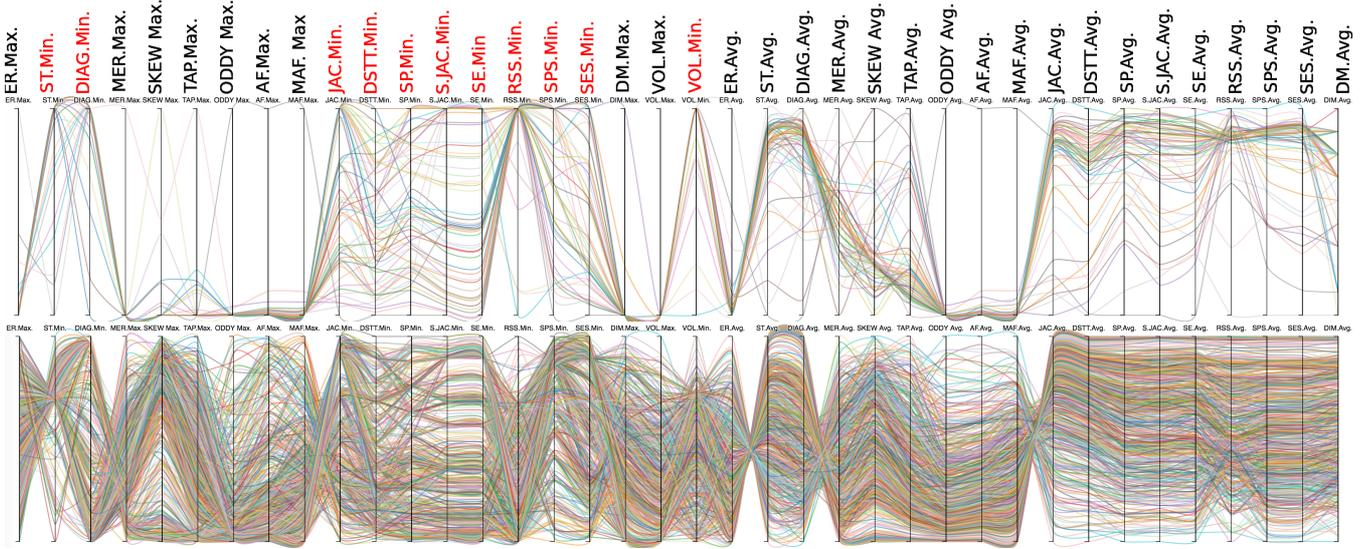
**Figure 2:** Top: Parallel coordinate visualizations of all the metric values of 67 crank hex-meshes by only controlling the minimum metrics with lower bounds and  $\uparrow$  trends (red labels). Bottom: the distribution of the 818 meshes from the second level perturbation.
