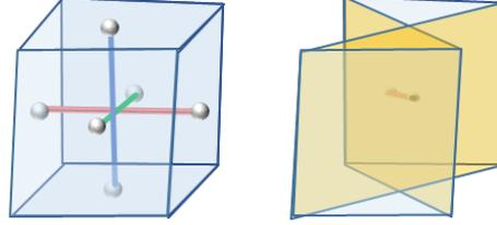
A hexahedron has three principal axes, each of which is pointing to the center of a face from the center of its opposite face (left of the figure). The cross-derivative of  $\vec{X}_{ij}$  is pointing from the center of one diagonal face to the center of the other one, where the diagonals of the two diagonal faces are on the two hex-faces of  $X_k$  (right of the figure).  $L_{ij}$  denotes the length of  $\vec{X}_{ij}$ .
