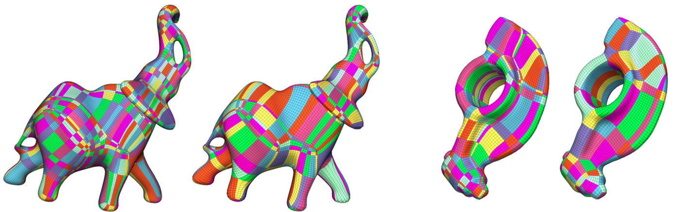
Fig. 3. Elephant, and Rockerarm-1 hex-meshes before (the left of each model) and after (the right of each model) optimization with our method. Original hex-meshes are obtained from [2]. Corresponding statistics are in Table 1 of the paper.
