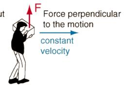
When an object is carried at constant velocity by a force which acts at right angles to the motion, no work is done on the object.
