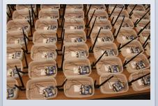
Twonet consists of 100 Opal nodes [5] with 2.4 GHz and 900 MHz radios deployed across four floors of an academic building. Similar to the way early sensor network testbeds helped advance research on wireless sensor networks, Twonet will enable new research on multiband radio communications and will enable new class of sensor network applications that utilize the powerful yet energy-efficient Cortex-M3 CPU architecture.
