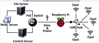
Twonet is inspired by earlier sensor network testbeds and uses the timetested three-tier architecture.
