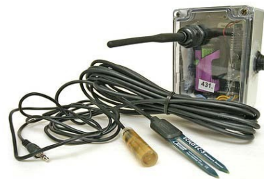
Figure 2: Our Gen-2 platform, based on the Telos mote.
