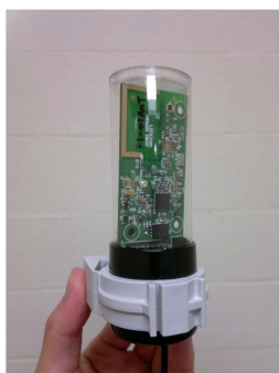
Figure 3: Our Gen-3 platform, based on our PCB design.
