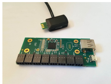
Figure 12: The CC430-based Toast and miniToast analog interface/multiplexer boards.
