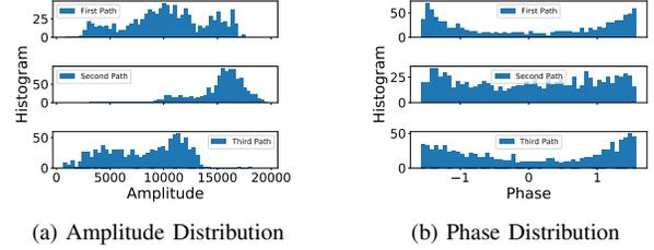
Fig. 5: Histogram of First 3 RMCs over 1000 Samples
