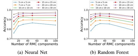
Fig. 4: Classification Accuracy using Raw CIR Information
