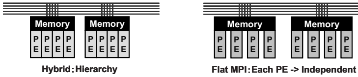
Fig. 1. Parallel programming models on SMP cluster architecture [1,2]
