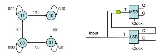
Two T flip-flops: one for the more significant bit and one for the less significant bit
