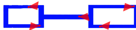
Figure 8: Configuration of cameras obtained by optimizing the cell coverage quality metric proposed by Janoos et al. 2007 for each cluster.(Janoos et al., 2007)
