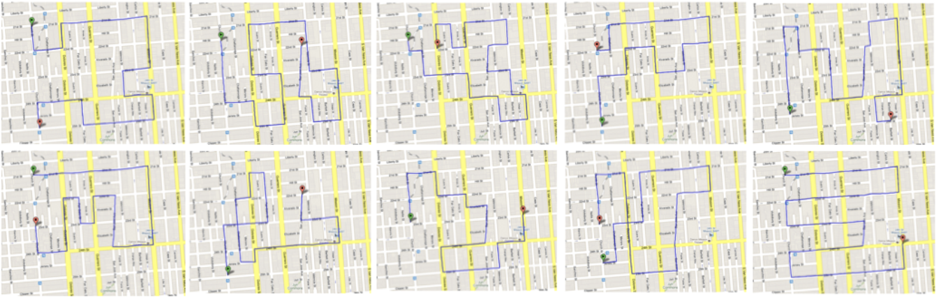
Figure 6: Moving paths of mobile vehicles. Each vehicle moves at a speed of \mathcal{N}(30, 5^2) in km/h. We generate 20 different moving paths including the opposite direction as well. All of 20 vehicles are moving over the networks while communicating with sensor nodes as in Fig. 5(a).
