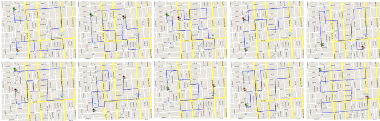
Fig. 12. Moving paths of mobile vehicles where each unique moving path is highly overlapped with others in part. Each vehicle moves at a speed of \mathcal{N}(30, 5^2) in km/h. We generate 20 different moving paths including the opposite direction as well. All of 20 vehicles are moving over the networks while communicating with sensor nodes as in Fig. 11(a).
