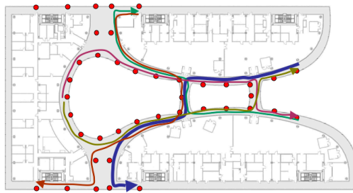
Fig. 9. 41 stationary sensors (marked with red circle) distributed over 65 \times 100 \text{ m}^2 and moving paths of mobile sinks in Clark building at Stanford University. 10 different moving paths including the opposite direction are explored while a mobile sink carries a sensor device and communicates with the networks.
