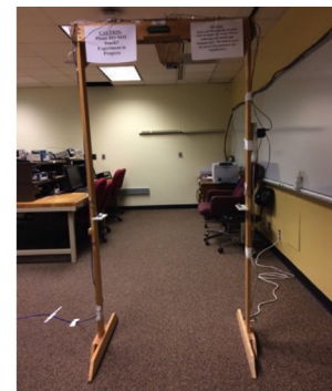
(c) Front view of the door frame with the ultrasonic sensors mounted.
