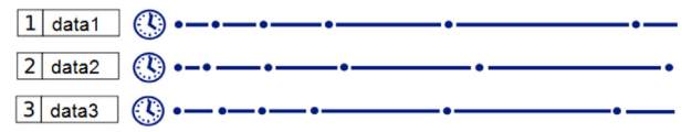
Fig. 2. Drip example. There are three values to be disseminated. Each value is independently associated with a Trickle timer. Each packet has a value (rectangles on the left side). Each dot represents when the timer fires and a message is sent.
